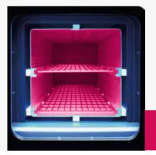
Neuster SW series sterilization systems utilize a RF plasma system to provide a residue free sterilization. The plasma system is activated during the sterilization process and enables the composition of hydrogen peroxide to water and oxygene molecules.
